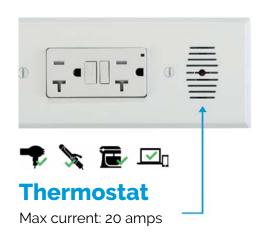
**Powering Outlets** are designed to power larger devices such as hair dryers, curling irons, stand mixers, phones, etc. These outlets incorporate an interlocking thermostat that continuously senses the ambient temperature. This interlocking safety feature will shut off power to the outlet if the surrounding air exceeds 120° F.
